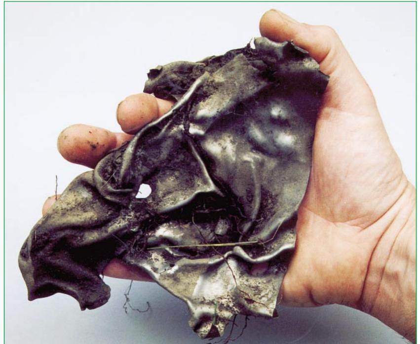
Mangled fragments of a B17's stainless steel oxygen tank.
