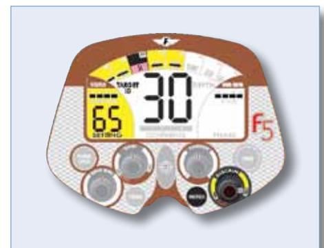
Once again the little panel on the left takes on its adaptive role as the F5's "universal indicator" whereby it temporarily displays the level of any adjustments made, which in this case is rejection.
