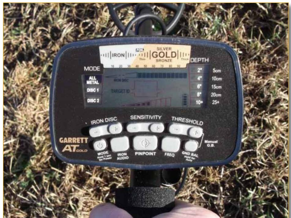
Fig.3. Disc 1 set up, with discrimination set on 40.
