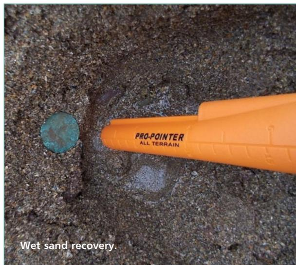
**Fast Retune for Mineralised Ground:** to tune out the detection of saltwater, wet sand or highly mineralised ground, hold the tip of the Pro-Pointer AT to the water, sand or soil and quick-press the On button for an instant retune.
