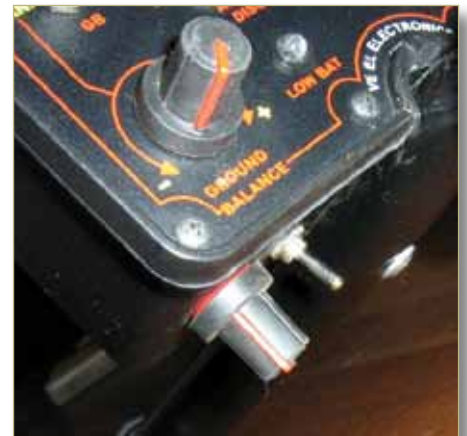
Fig.2. Frequency Adjust control and the Turbo Boost switch.
