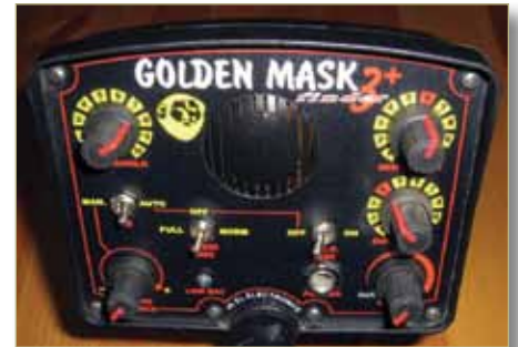
Fig.1. Control box layout of the Golden Mask GM3+.
