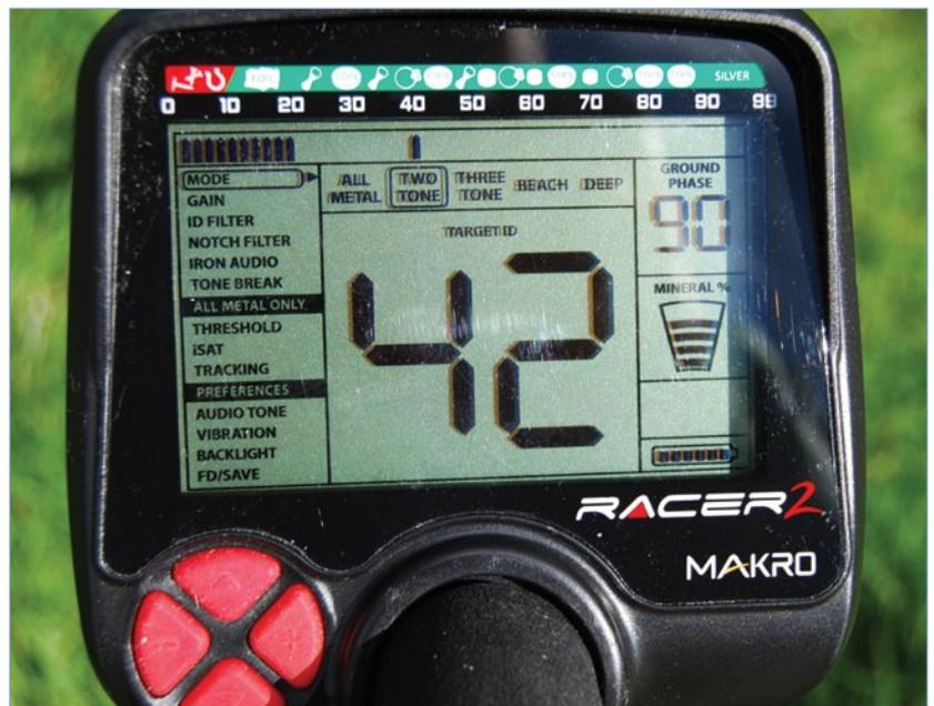
Meter shows cursor, Target ID, Ground Phase and Mineral Content.
