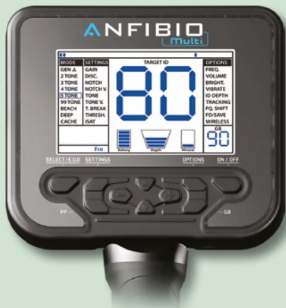
Figs.1 & 2. Control box display of the Anfibio Multi detector.
