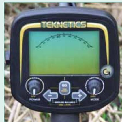
Fig.2. G2 control panel and display.
