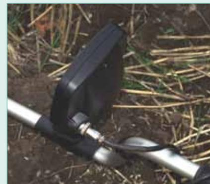
Fig.3. Underside of the control box showing cable connection.
