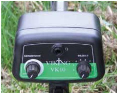
Fig.2. The simple control panel of the VK10.
