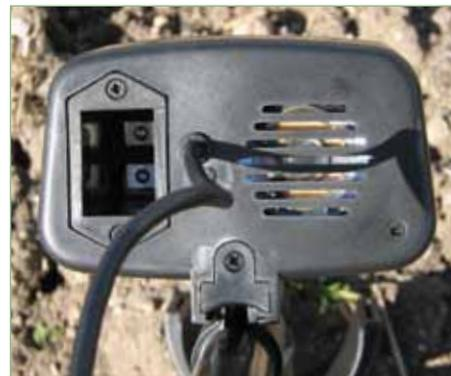
Fig.4. The battery housing and speaker.
