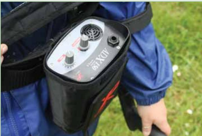
Fig.7. The waterproof hip-mounted control box pouch.
