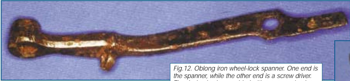
Fig. 12. Oblong iron wheel-lock spanner. One end is the spanner, while the other end is a screw driver. The device is also provided with a suspension loop.
