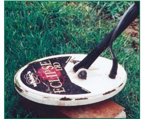
The 9.5in concentric and 10in x 5in elliptical coils used in the test.
