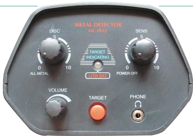
This is marked "VOLUME" and works simply as described. It allows audio to be set at a level that is comfortable to the user's hearing. Next to the volume control is a red push button that is labelled "TARGET". This helps to pinpoint in on a specific metal find.
