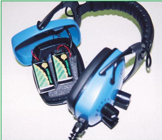
The simple controls of the Headhunter Wader.
