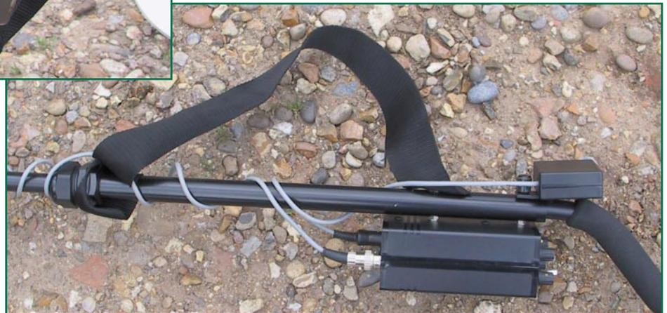
GND control should be initially set to the pre-set position (6-7). At these settings the smaller pieces of iron, silver paper and other trash items will be either rejected or identified. When working on the beach or other areas where junk contamination is a problem, the Reject control should be raised to a higher level.
