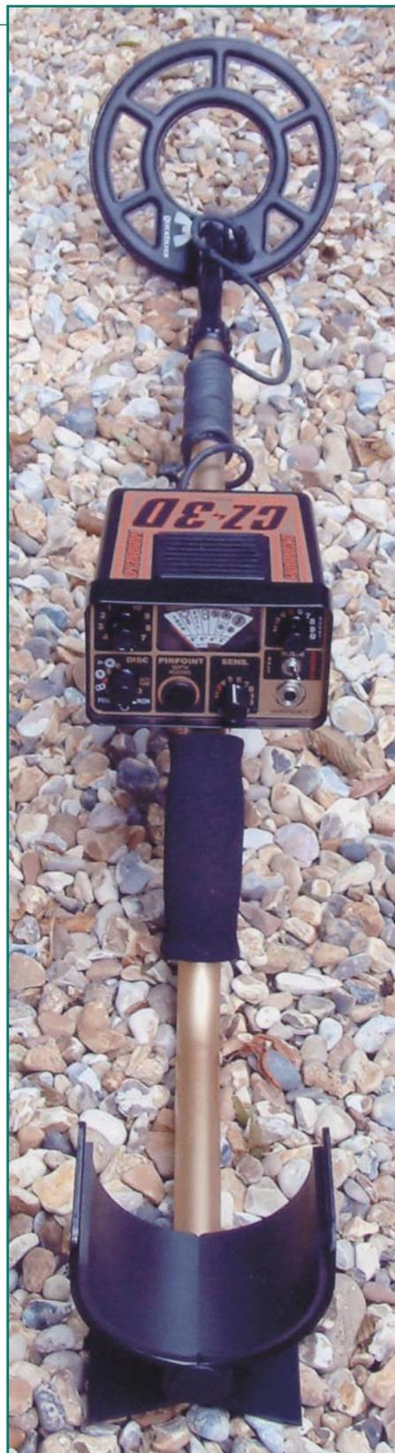
lowering the coil to the ground. Rotate the ground control from the 10 position until you hear an audio tone; back it off until the tone disappears, release the pinpoint button and you are ready to search.
