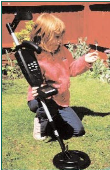
at all relating to build quality and performance. When passed over the coins on the surface a small target indicator arrow positions itself beneath a selection of illustrations. Two pence coins register below the illustration of a 5 cents coin. Checking the lawn revealed another "5 cents target" buried 6in down, and - you guessed it - it was another 2p.
