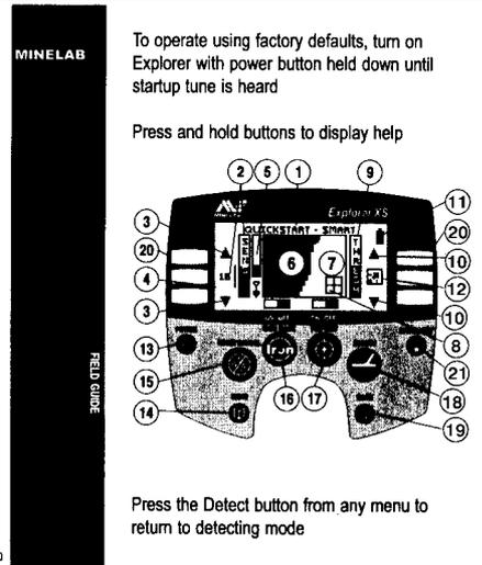
To operate using factory defaults, turn on Explorer with power button held down until startup tune is heard
