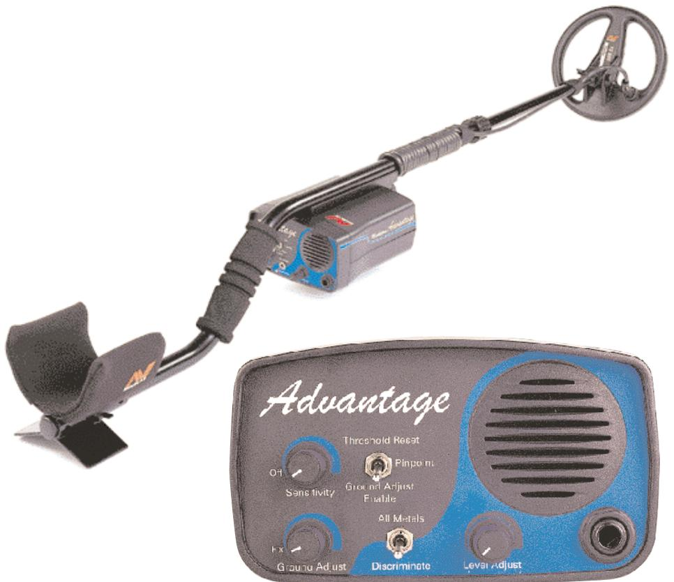
Sensitivity is combined with the On/Off knob and should be turned as far clockwise as it can go until the detector begins to chatter. This might vary from site to site, but in the main you will find this detector extremely quiet until it finds a target.
