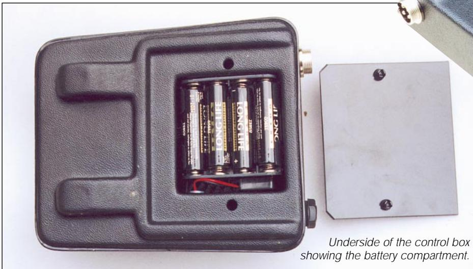
Underside of the control box showing the battery compartment.
