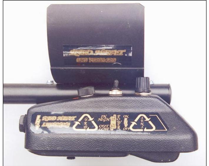
*When the control box is fitted under the arm-rest access to the controls can be awkward.*
