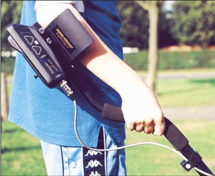
*The coil lead is in an awkward position.*
