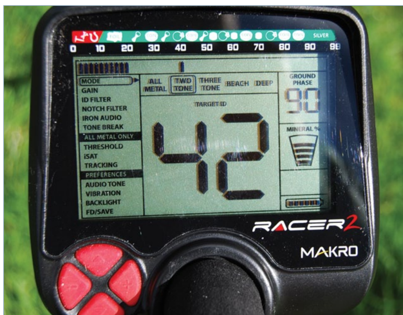
Meter shows cursor, Target ID, Ground Phase and Mineral Content.
