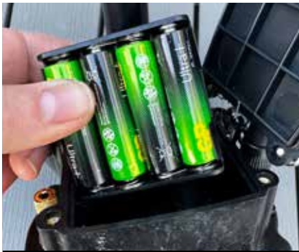
Fig.4. The 6MXi battery compartment.
