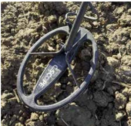
Fig.5. The 6MXi 20 x 28cm 2D elliptical coil.
