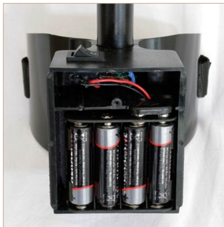
Fig.2. Battery housing and on/off switch.
