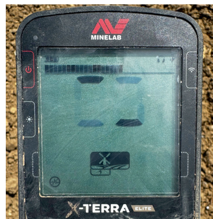
Fig.9. The rolling Noise Cancel on the X-Terra Elite picking one of 19 available channels.
