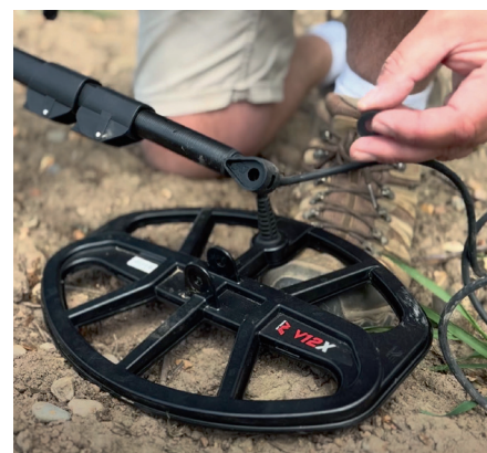
Fig.10. Removing the V12X coil to change to the smaller V8X in long grass.
