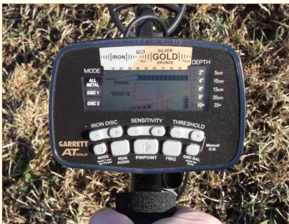
Fig.2. Meter with the All Metal settings on.
