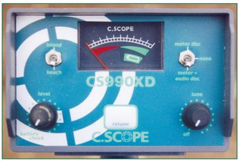
Fig.2. The CS990XD's control panel.
