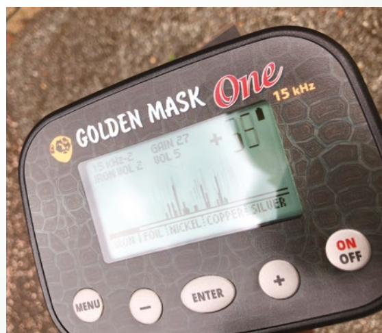
The trash signal on the GM15 display.
