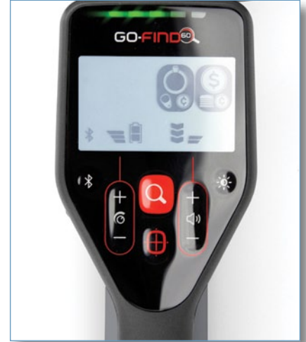
The Minelab Go-Find 60 LCD screen.
