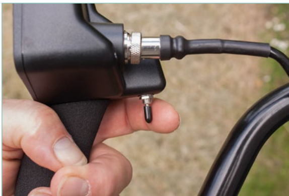
Fig.6. Trigger Switch for Pinpoint Mode and Ground Cancel.
