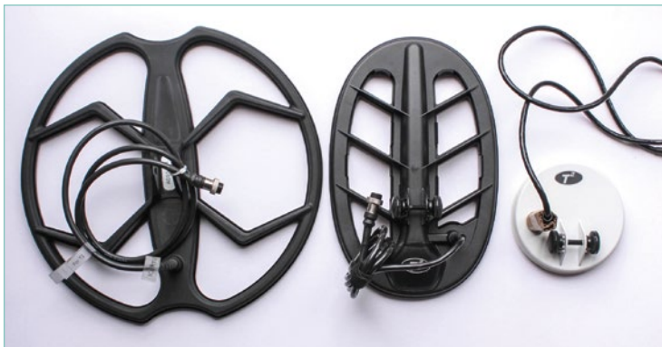
Fig.2. The three search coils used for the test - 11 inch, 13 inch and 5 inch.
