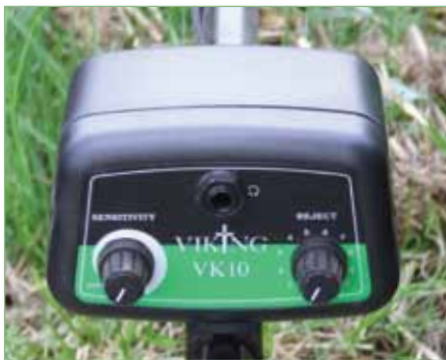
Fig.2. The simple control panel of the VK10.
