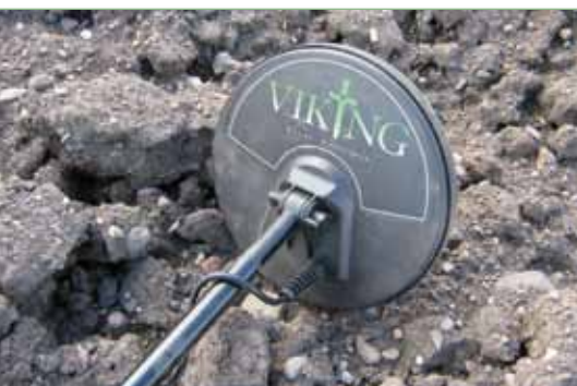
Fig.3. The 8 inch waterproof search coil with scuff cover fitted.
