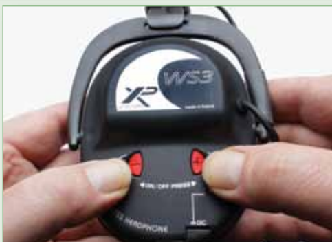
Fig.8. Switching on the headphones by pressing both buttons.
