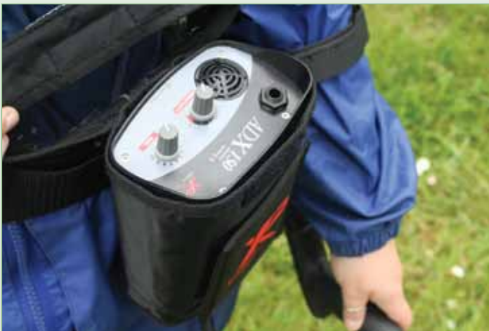
Fig.7. The waterproof hip-mounted control box pouch.
