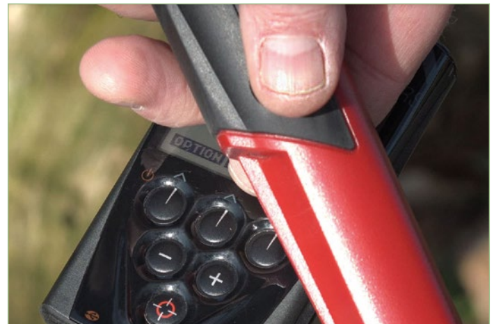
Fig.7. Press and hold pressure pad for around 8 seconds to finalise the pairing procedure.
